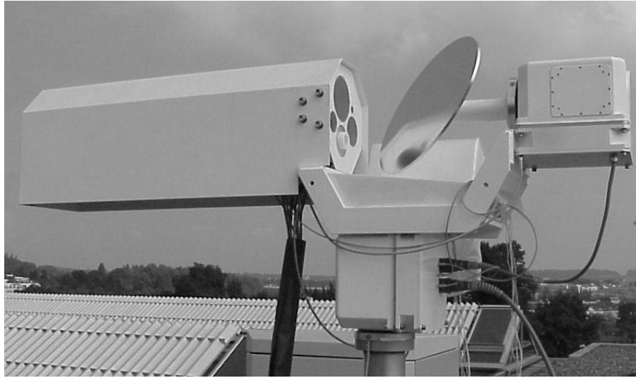
Figure 5 - ASMUWARA in operation in Bern. The openings of the 4 horns appear as grey disks at the left of the rotatable mirror, while the IR radiometer looks through the white cylinder below the largest horn.
