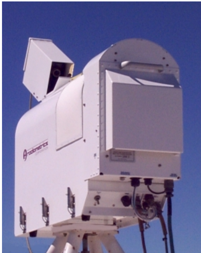
Figure 1. Temperature, water vapor, and liquid water profiling radiometer.
