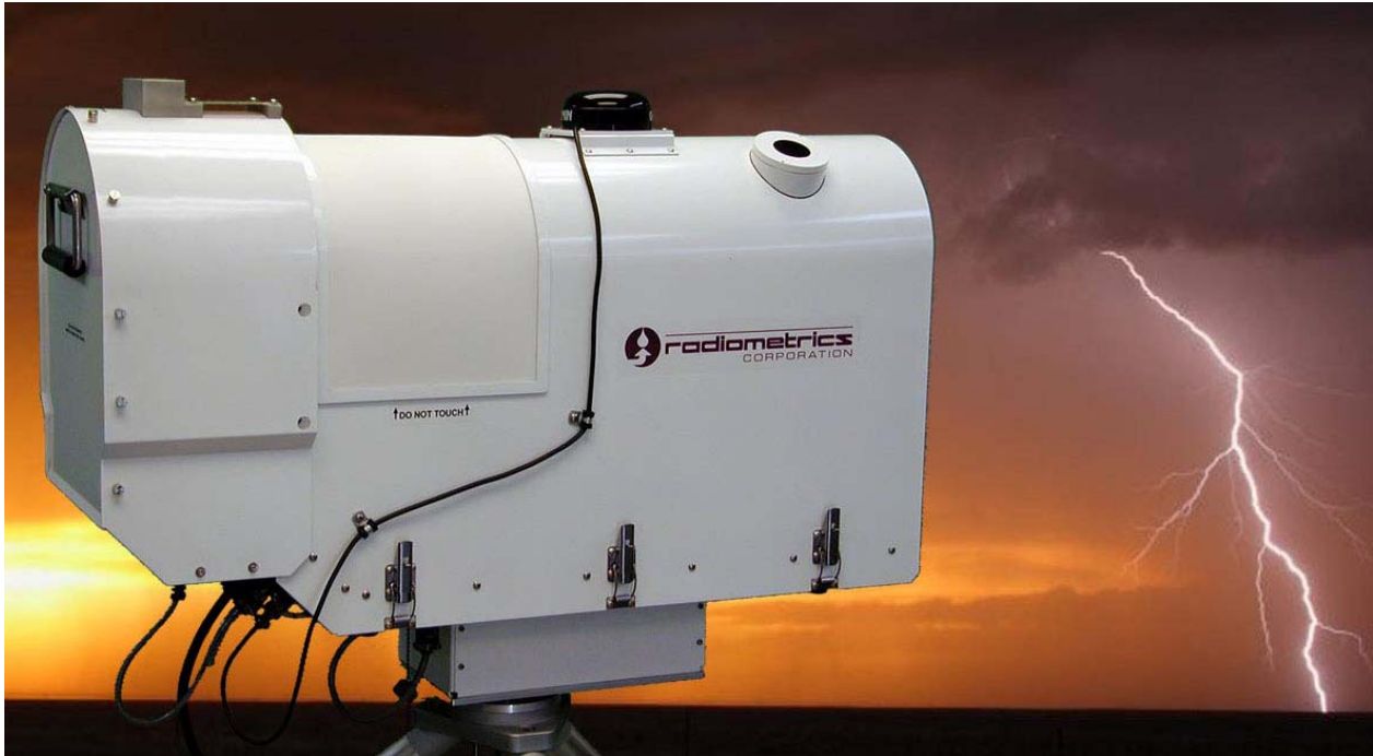
Figure 1. Radiometrics MP-3000A Microwave Profiler directly detects liquid water (supercooled or above freezing) that is essential for weather modification.
